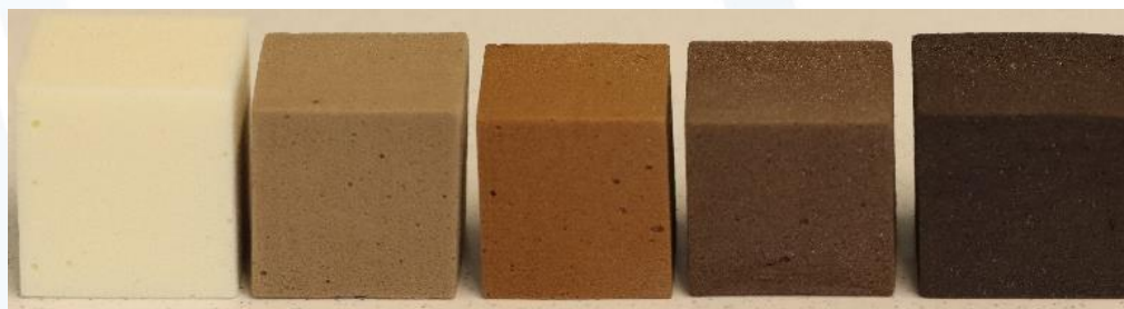
Specimens of rigid polyurethane foams containing increasing amounts of furfural-derived polyols
