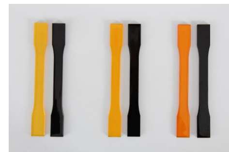
Reference (left) and lignin-based (right) specimens of 2K polyurethane adhesives
