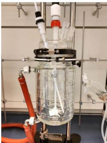
5L jacketed glass reactor for upscaling of chemical syntheses
